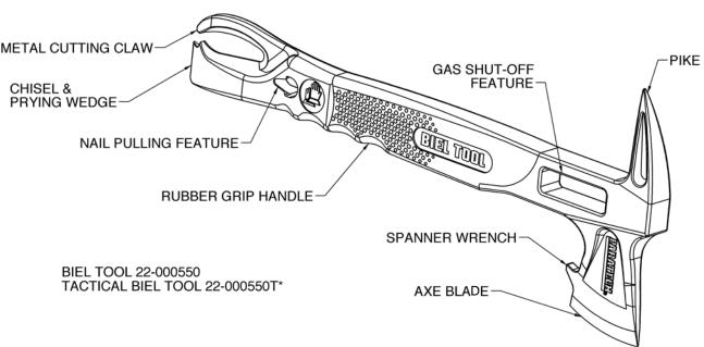
The Biel Tool is designed to be an ergonomic, light, wearable (using available Sheath or Tactical Pouch) multi purpose fireman's personal tool that can be employed instantly without any preparations and used for multiple purpose forcible entry and rescue. The Biel Tool complies with SAE International Aerospace Standard AS5402 and NTSB Crash Ax e requirements.
